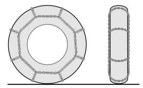
Figure I (a) Inappropriate ladder snow chains
